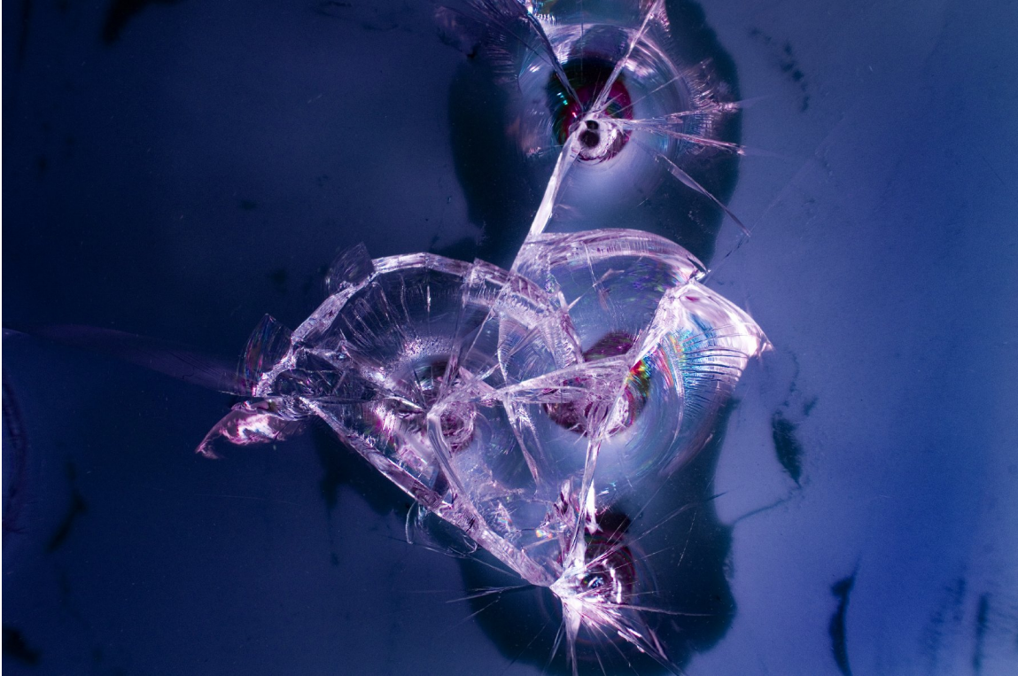
Figure 34 A base view of the same main cluster of impacts in glass with a clay coating shown in figure 33. Note the size of the cone base to crater ratio. The circular shadow area in the background indicated clay being pulled away from the glass and is more proportional to crater/HC features in rock.
