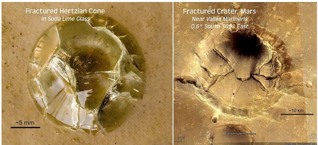
Figure 21 Above left is a Hertzian cone created by a mid-velocity impact. On the right is an unnamed fractured crater with similar features. HC's vary in fragmentation with the velocity and mass of the projectile. Such should hold for planetary impacts.
