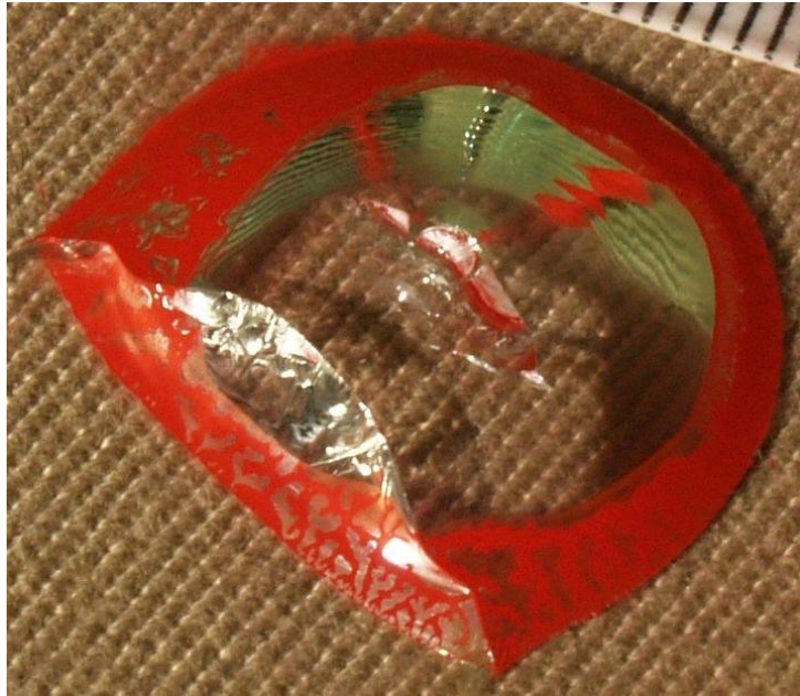
Figure 27 Above is a sample of a Hertzian cone in situ with overburden intact. Dye was forced into the HF around the cones to simulate volcanic intrusion. The POI can be seen in the center of the shield cone with a winged crack along the base directly below.
